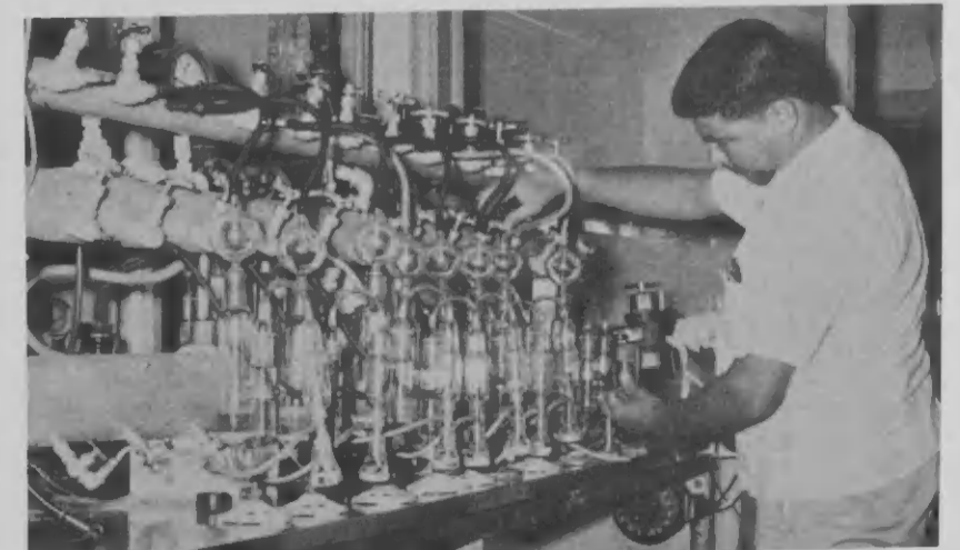
THE LAMP test for determining sulphur in gasoline is being run by Juan Ras.
